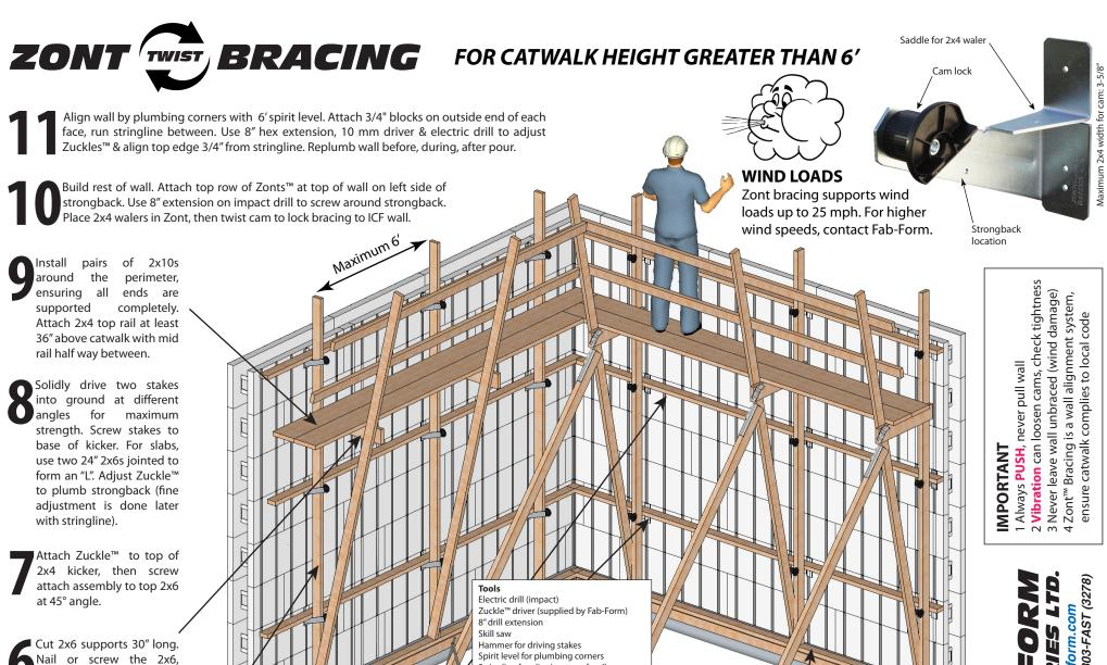
strength. Place STRAIGHT 2x4 strongbacks on right side of Zont™, toe-nailing base to 2x4 plate. Tighten cam counter-clockwise to
